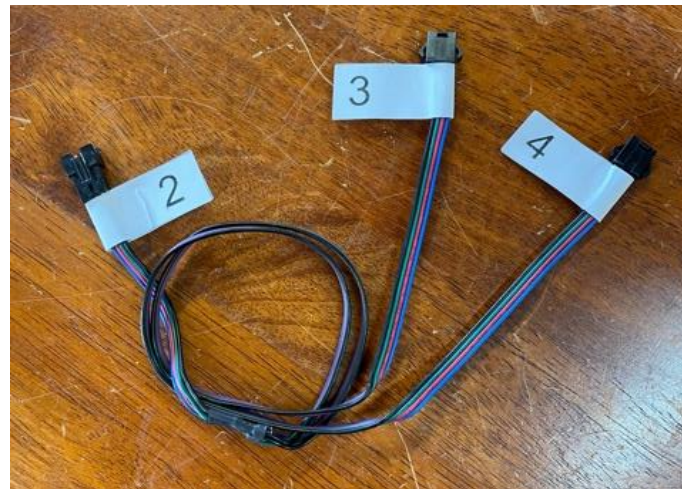
1 to 2 Splitter Terminals labeled
